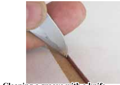
Cleaning a groove with a knife
